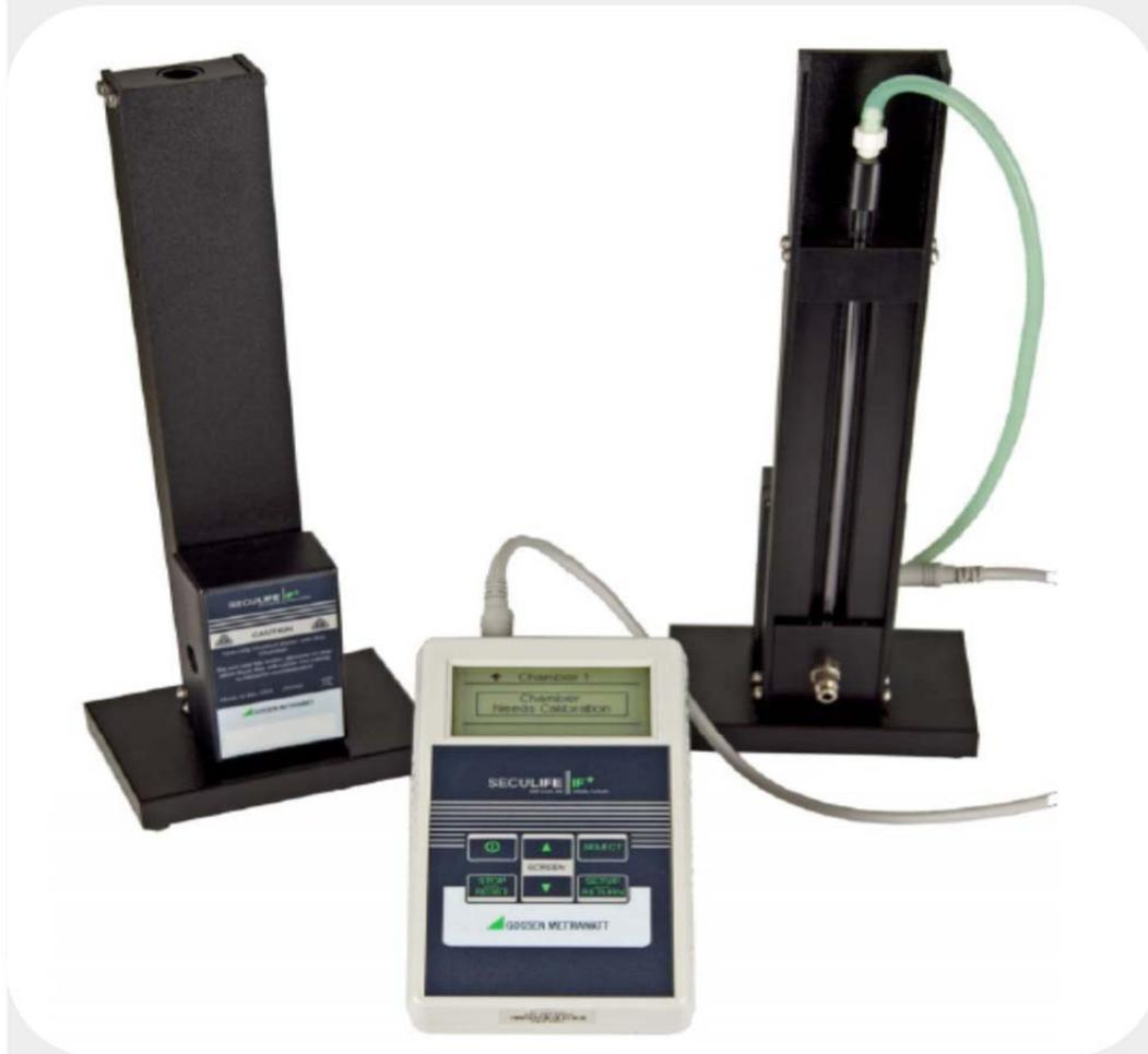
The SECULIFE IF+ is a microprocessor based high precision Infusion Pump Analyzer (IPA). It tests the flow of intravenous (I. V.) infusion pumps. The flow rates are displayed in milliliters per hour. Simultaneously the unit can test two volumetric pumps for output flow rate using two volumetric chambers.
